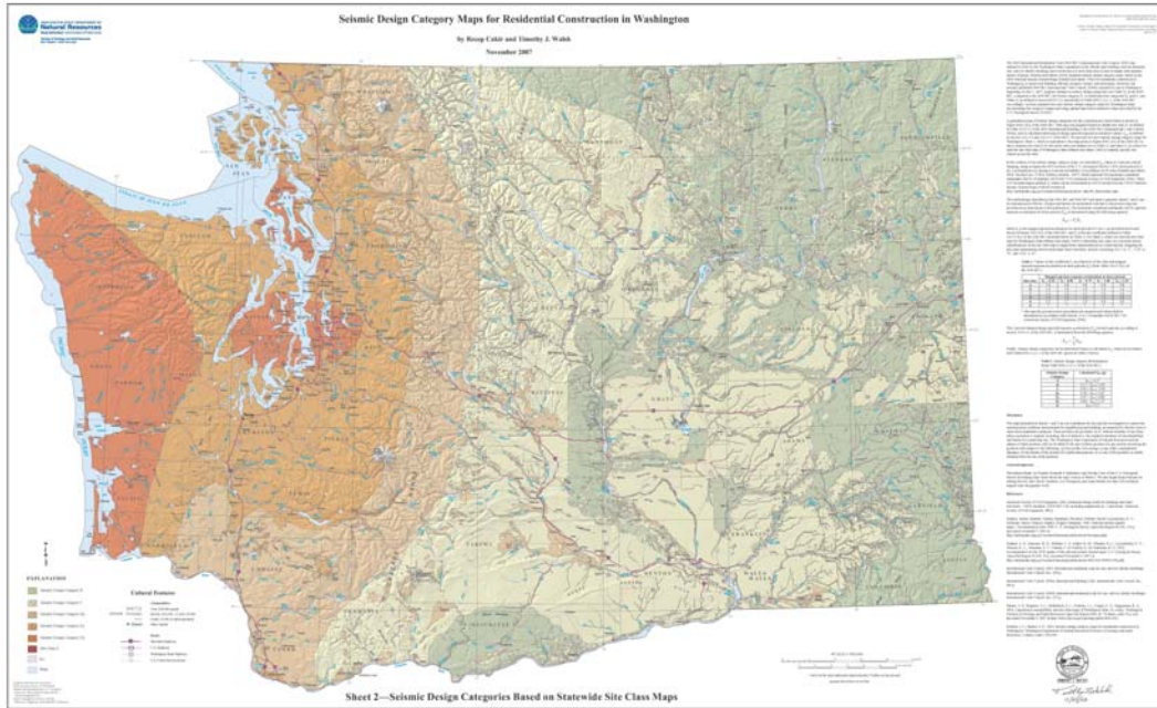
Figure 1. Example of a seismic design category map for residential construction, produced by the Division. Shallow seismic surveys are required to make these maps.
