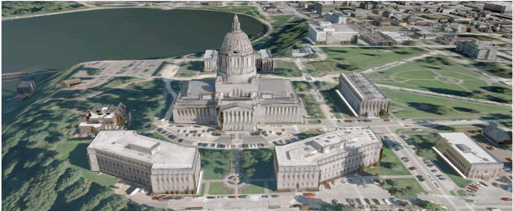
Stop 1. The Capitol campus is built on loose sand and silt deposited at the end of the last ice age. This material tends to amplify earthquake ground motions. Part of the campus (for instance, a gully under where the greenhouse now stands) also has loose fill placed on it, which further amplifies ground shaking.
