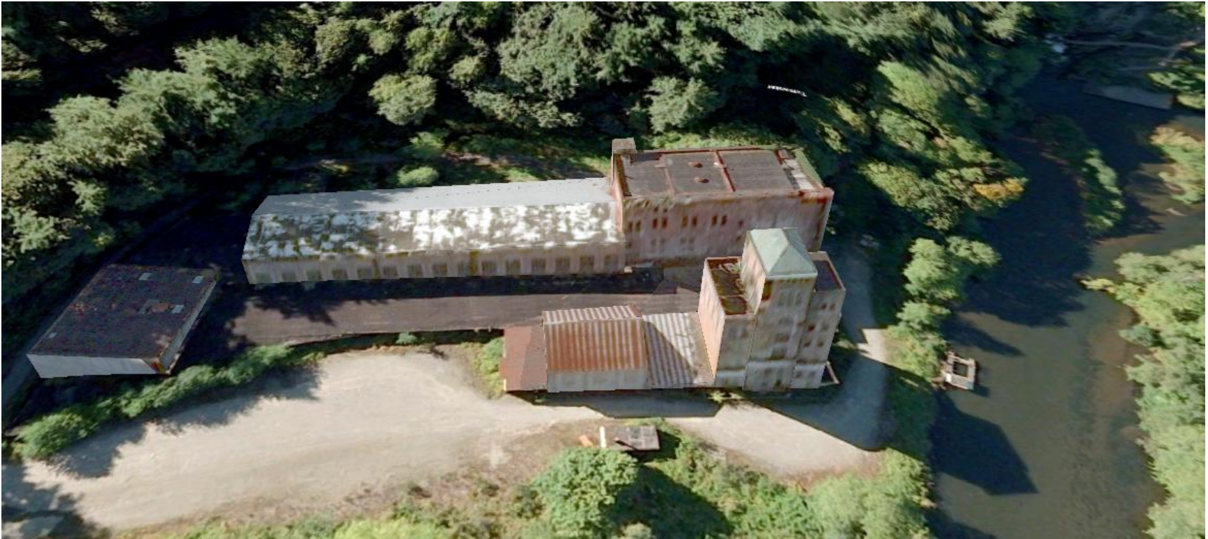
Stop 2. Old Olympiabrewery, built of unreinforced masonry in 1906. Although this building is dilapidated, it was not damaged in the Nisqually earthquake. This building is founded on bedrock, the basalt of the Crescent Formation which make up the Black Hills to the west of here.
